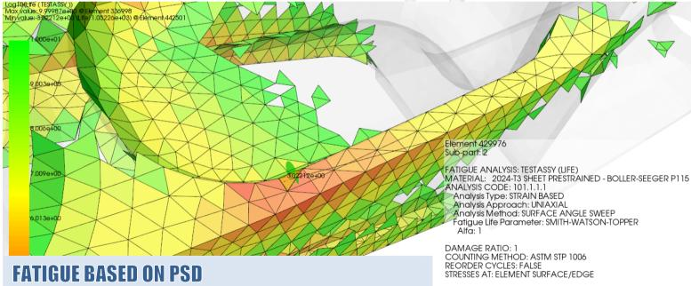
Other than conventional methods for fatigue calculation based on spectra in the time domain, also fatigue due to vibration can be assessed, i.e. in the frequency domain.
