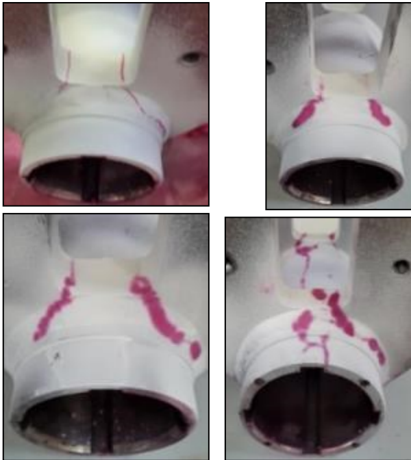
Crack position highlighted by PT test.
